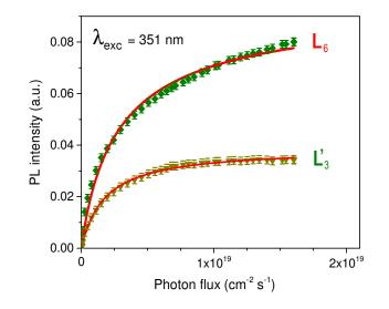
Figure 4: PL intensities measured at 10 K as a function of excitation flux for line  $L_6$  from the isolated Er optical centers and  $L_3$  from the defect-related Er optical centers, under band-to-band excitation ( $\lambda_{exc} = 351.1$  nm).
