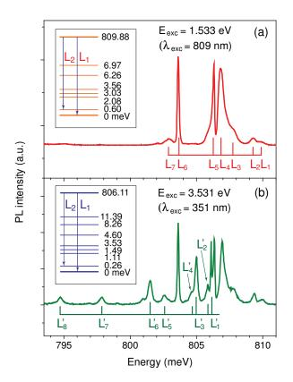
Figure 1. PL spectra of the GaN:Er epilayer of 0.5  $\mu$ m thickness at 1.54  $\mu$ m within the  ${}^{4}I_{13/2} \rightarrow {}^{4}I_{15/2}$  transition as measured at 15 K under (**a**)  ${}^{4}I_{15/2} \rightarrow {}^{4}I_{9/2}$  resonant (1.533 eV or 809 nm), (inset) energy level diagram of the isolated Er optical center, and (**b**) non-resonant or band-to-band (3.531 eV or 351.1 nm) excitation, (inset) energy level diagram of the defect-related Er optical center.
