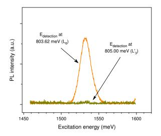
Figure 2. A comparison of PL excitation spectra around 1.533 eV (809 nm) detected at  $E_{detection} = 803.62$  meV (1542.83 nm) for line L<sub>6</sub> and  $E_{detection} = 805.00$  meV (1540.19 nm) for line L'<sub>3</sub> reveals a low number of optical centers for the L' center.
